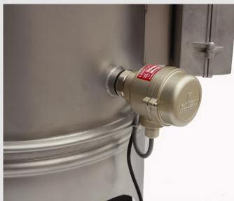
料位开关安装在真空料斗上，用于控 制循环批次上料 Level switch installed in vacuum hopper for control of batch loading cycle
