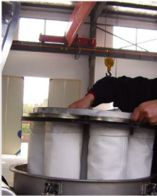
过滤单元可作为整体拆卸， 使得布袋维修更换和物料更 换更方便 Filter removed in one piece for easy product discharge
